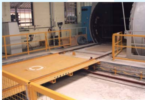
This traversing platform manufactured for Aerostructures takes product to and from their autoclaves
