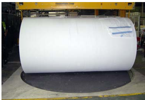
A Ø3.6m 5 tonne capacity air-film turntable provides Georgia Pacific with a low-friction means of manually rotating reels of paper
